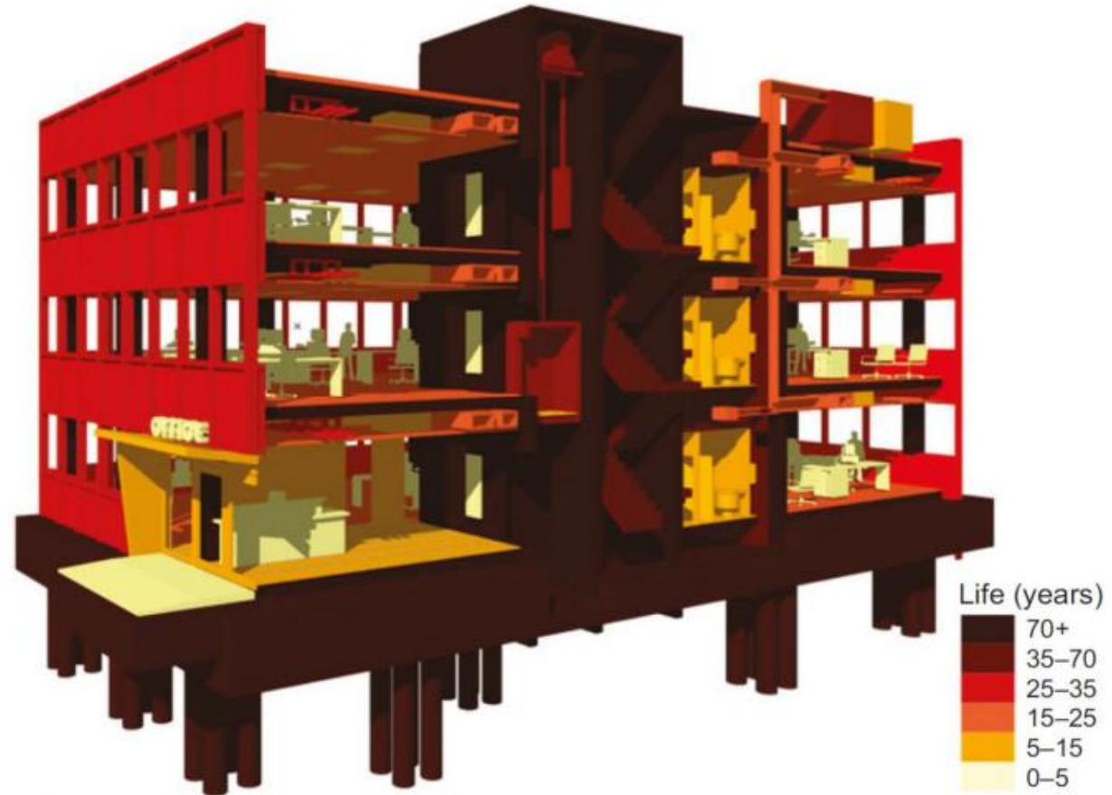
Figure 3. Average lifespans of components within an office building. Source: Sturgis Associates LLP (2009)
